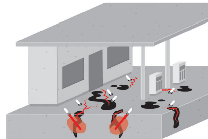
Repair of oil-contaminated cracks
