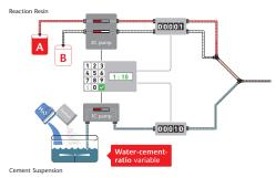
The cement used is the one available at the working site; it is adjusted as usual (water-cement-ratio), if necessary, by additives (superplasticizer, dispersion aids, anti-segregation aids, accelerator, retarder) according to the needs of the construction site, the application and the desired performance
