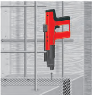
Installation of WEBAC® Bentonite Swelling Tape with WEBAC® Fastening Grid , mechanical fastening
