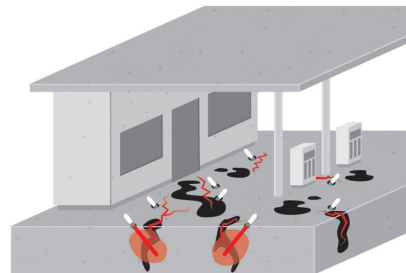
Repair of oil-contaminated cracks
