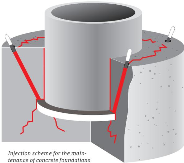
*Injection scheme for the maintenance of concrete foundations with WEBAC packers and WEBAC injection material*
