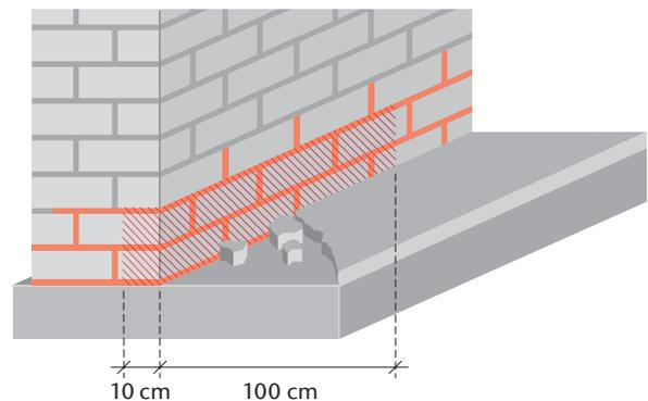
The material consumption depends on the pore and cavity volume of the masonry.
