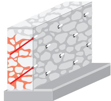
Filling of cavities/voids in masonry
