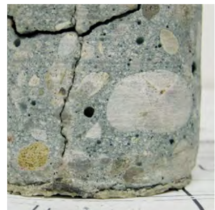
Drill core removal: Determination of voids, crack progression, moisture condition and contaminations
