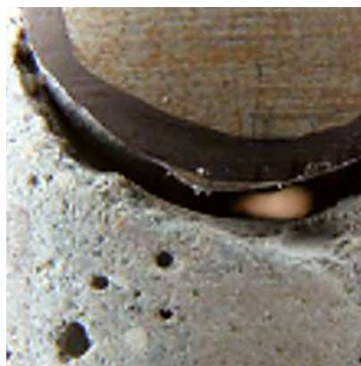
Drill core removal: Determination of voids, crack progression, moisture condition and contaminations
