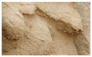
Fig. 6: Example of a gel curtain after injection
