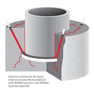
WEBAC Epoxy Injection Resins and special solid polyurethane resins are especially designed for the postconstruction repair of concrete parts such as foundations exposed to extreme loads.
